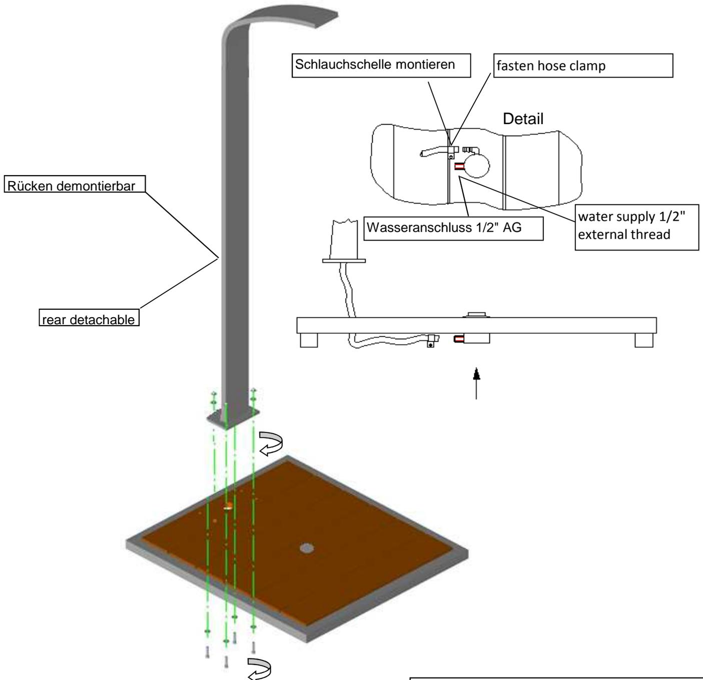
Transport may have loosened your shower's screw and bracket connections. If the shower leaks after first installation, please unscrew the rear and fasten the connections.
